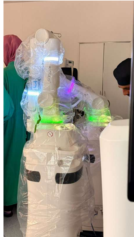
Figure 1: CMR Versius robotic arm docked for robotic-assisted cholecystectomy
